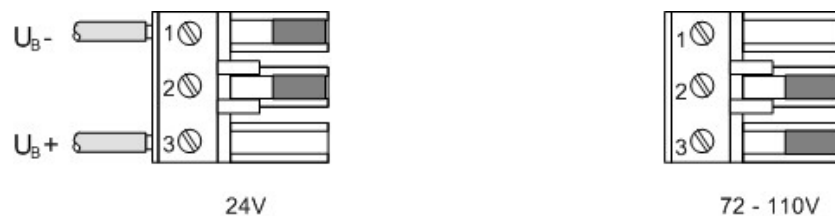
Figure 7 SV5 Terminals and coding of connector X1
